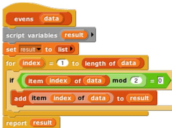
In this script, we first create a temporary variable, then put an empty list in it, then go through the items of the input list using the **add ... to (result)** block to modify the result list, adding one item at a time, and finally report the result.
